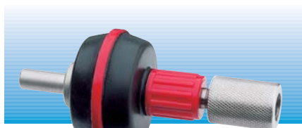
FK 1 Flexible coupling Required for stirring tasks using glass stirring rods. The flexible coupling compensates for any structural variances.
